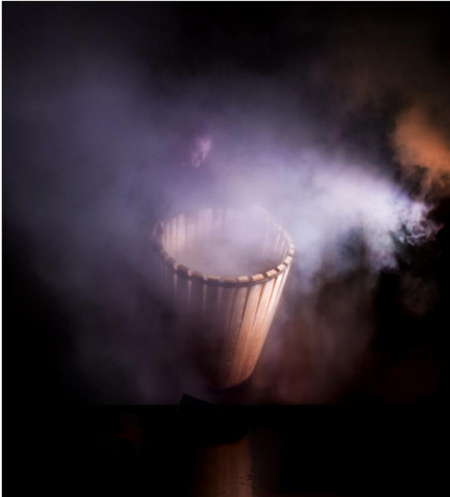
To shape the barrels Tonnellerie Ermitage uses a unique technique of bending using steam.
